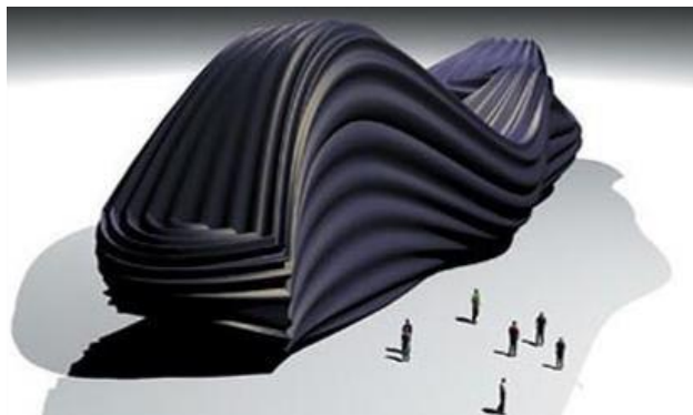
Figure 12: The elongation and contraction for pneumatic strips converts the digital information into motion and changes the form of the pavilion [19].
