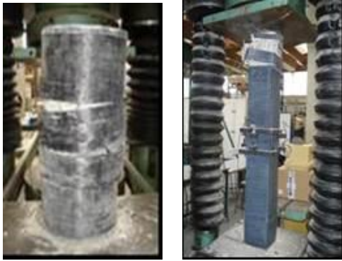
Fig. 2: Failure of CFRP confined specimens
