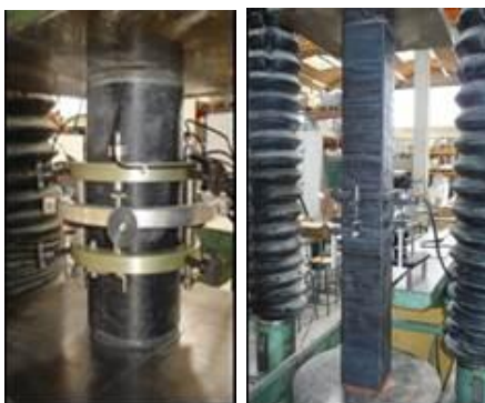
Fig. 1: Test setups for circular and square columns
