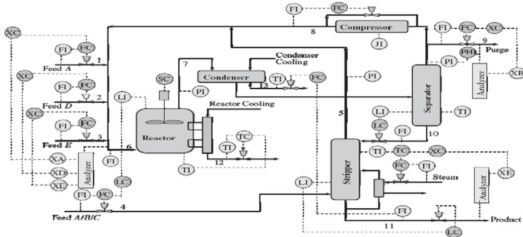
Fig. 1 Tennessee Eastman challenge process schematic diagram
