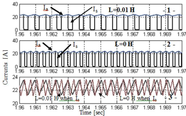
Fig 4 shows Ia and Is with and without smoothing coil
