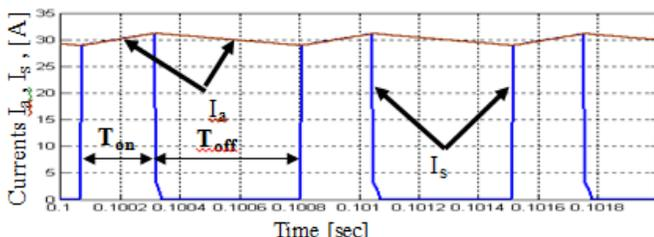
Fig 6 illustrates signal form at starting time, during chopper connected stage so Ia increase and Ia decrease during chopper cutoff.
