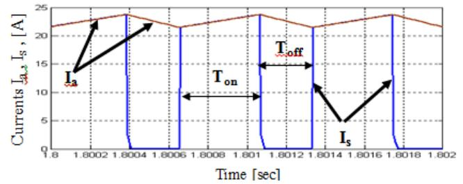
Fig 7 illustrate current signal form during loaded motor operation (Choppers Period connecting is increased)
