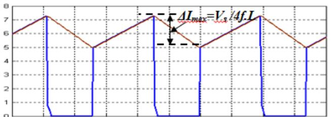
Fig 5 illustrate current signal form during unloaded motor operation
