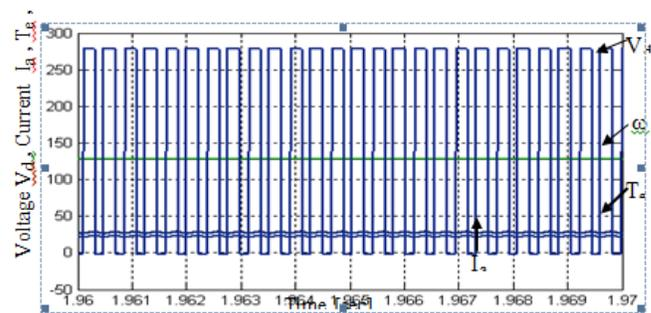
Fig 9 shown signal shape for Te, Ia, ω, Vd when  $L=0H$
