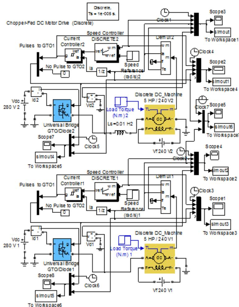
Fig. 2 block diagram to simulate the driving system when chopper supply by battery
