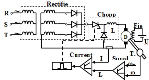
Fig. 1 General structure of the chopper fed Dc motor
