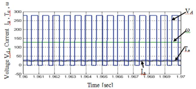
Fig 8 shown signal shape for Te, Ia, ω, Vd at  $L=0.01H$
