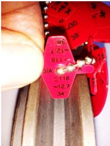
Fig. 8 The application of a V-Pulley gauge to measure a V-Pulley groove
