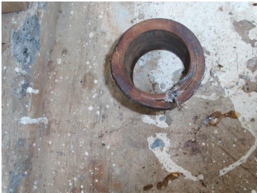
Fig. 3- Worn out bushing
