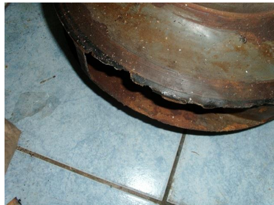
Fig. 7(b)- Damaged impeller due to cavitation
