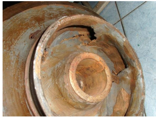
Fig. 7(a) – Damaged impeller due to cavitation
