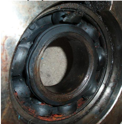
Fig. 2- Corroded and damaged bearing
