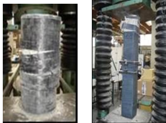
Fig. 2: Failure of CFRP confined specimens
