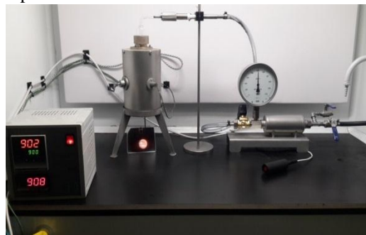
Fig.1. Godbert Greenwald Apparatus (ASTM1241).
