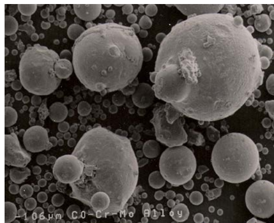
Fig. 2 Coarse Co-Cr-Mo powder with inferior surface finish
