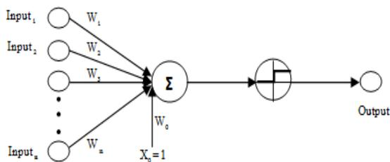
Fig. 3 Structure of a perceptron
