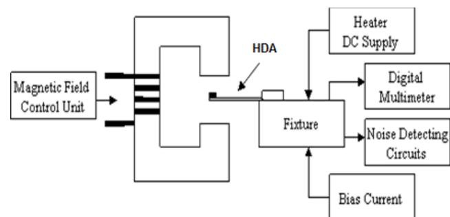
Fig. 1 The structure of Quasi-static test
