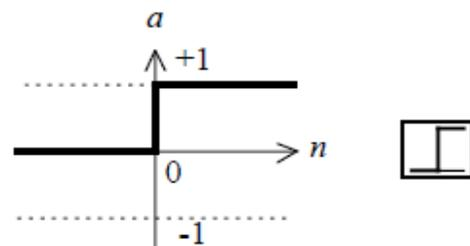
Fig. 5 Hard limit transfer function
