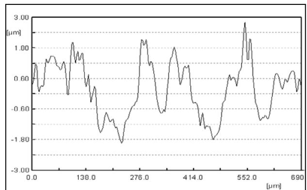
b) An example of measured surface roughness
