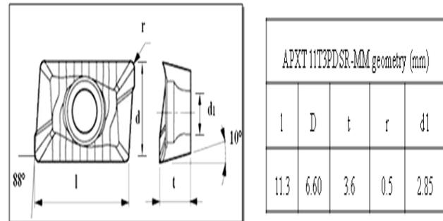
Fig. 1 Geometry of KORLOYS carbide insert
