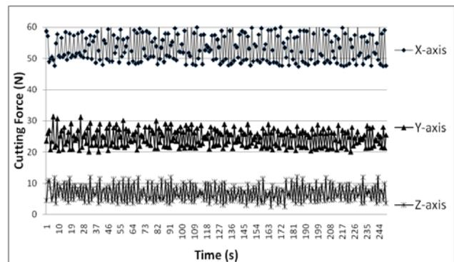
a) An example of measured cutting forces in X, Y and Z-axis directions
