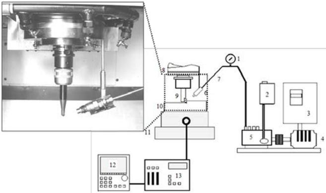
Fig. 2 Thin pulsed jet system experiment set up: 1- pressure gauge; 2- fluid tank; 3- variable speed control drive; 4- electric motor; 5- injection pump; 6- nozzle; 7- steel pipe; 8- spindle; 9- insert tool holder; 10- workpiece; 11- Dynamometer 12-charge amplifier;13- oscilloscope)
