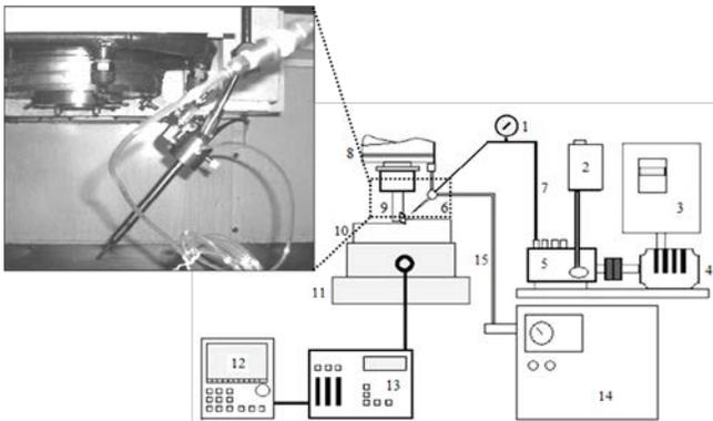
Fig.3. Fluid atomizer system experiment setup: 1- pressure gauge; 2- fluid tank; 3- variable speed control drive; 4- electric motor; 5- injection pump; 6, mist coolant; 7, steel pipe; 8- spindle; 9, insert tool holder; 10,- workpiece; 11- Dynamometer; 12- charge amplifier; 13- oscilloscope; 14- air compressor; 15- air stream supply
