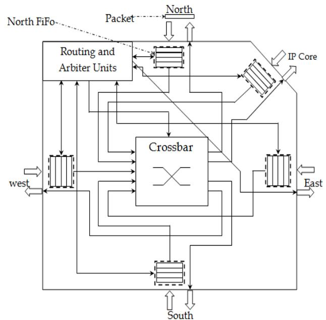
Fig. 4 Router architecture.
