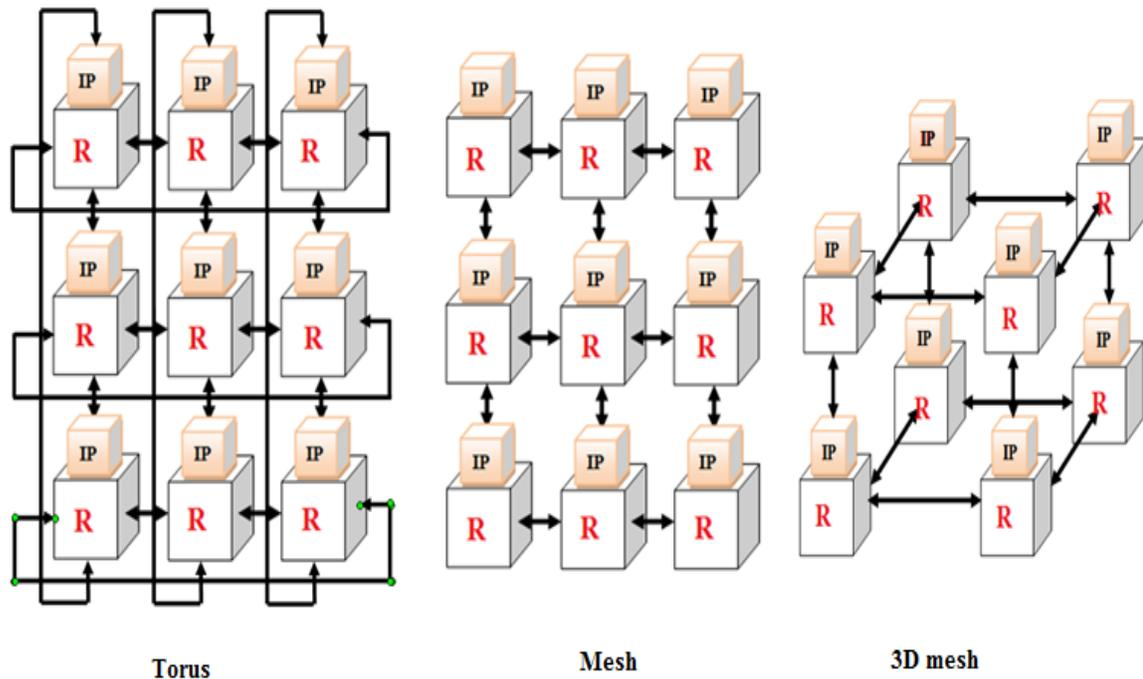
Fig. 3 Network on chip topologies.
