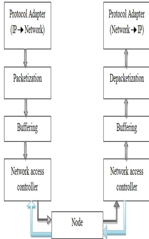
Fig. 2 Network Interface architecture.
