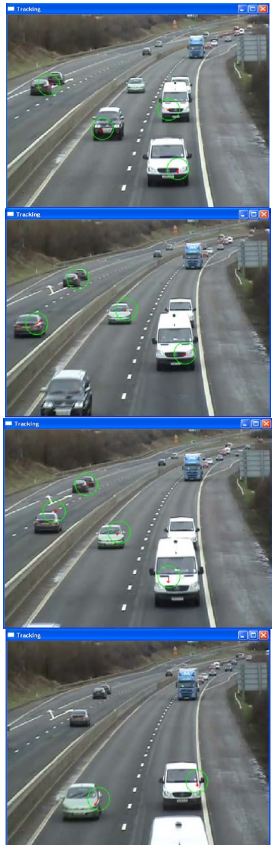
Fig. 5 Motion tracking and velocity estimation for many cars
