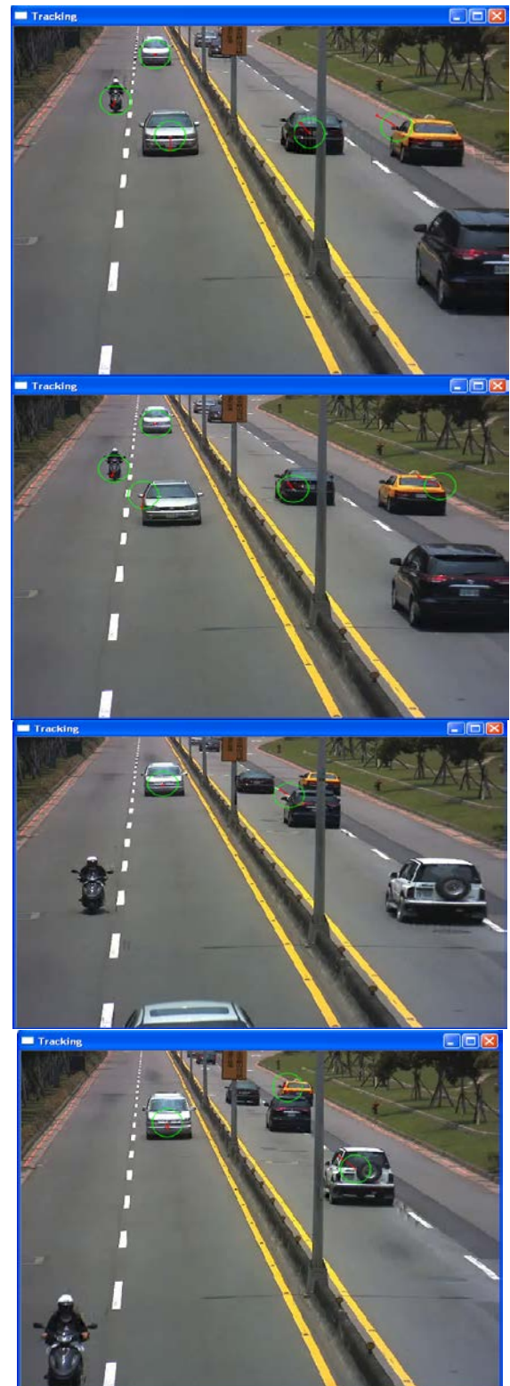
Fig. 3 Motion tracking and velocity estimation with occlusion effect at separator
