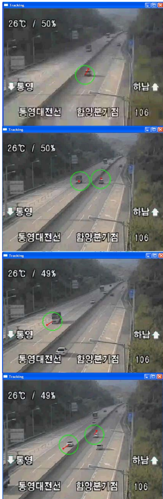
Fig. 6 Motion tracking and velocity estimation in bad quality video file
