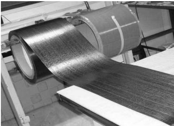
Fig. 1 Carbon fibers pre-impregnated epoxy resin unidirectional ply
