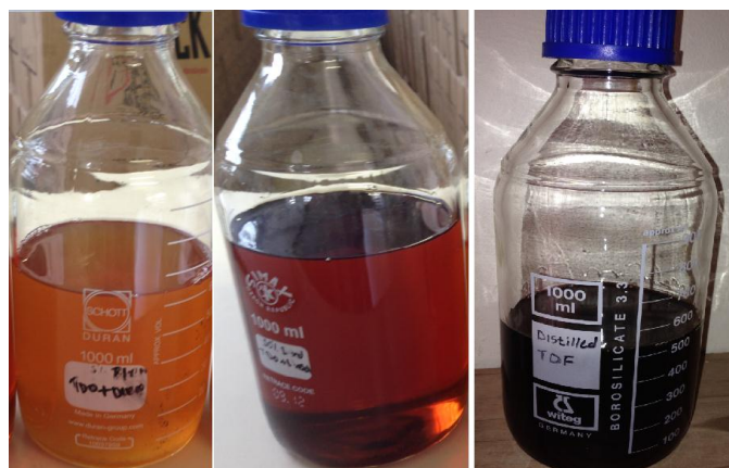
Fig. 2 Distilled rubber oil at 150, 200 and 250°C from left to right
