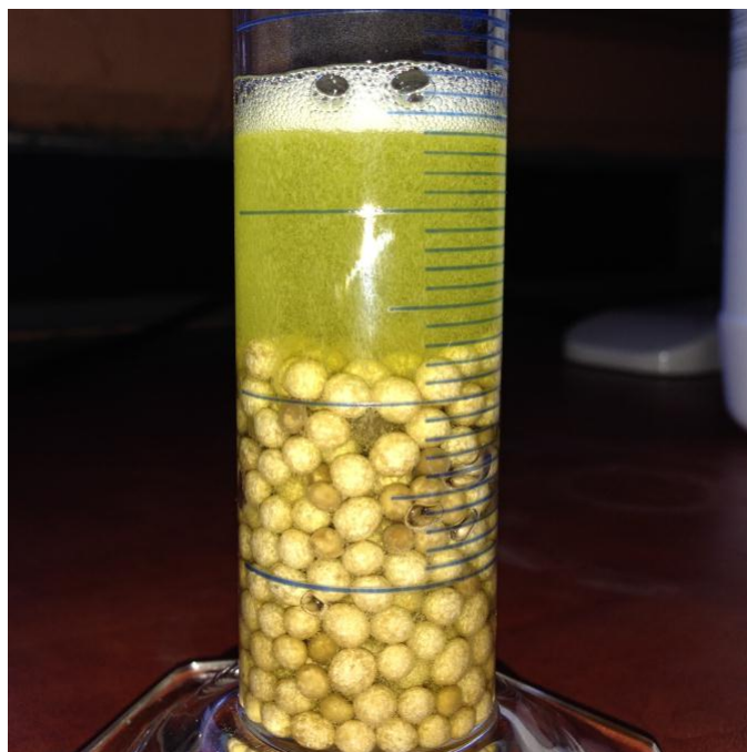
Fig. 5 Distilled rubber oil undergoing molecular filtration
