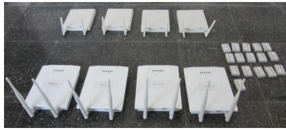
Fig. 3 RF CODE transmitters and receivers
