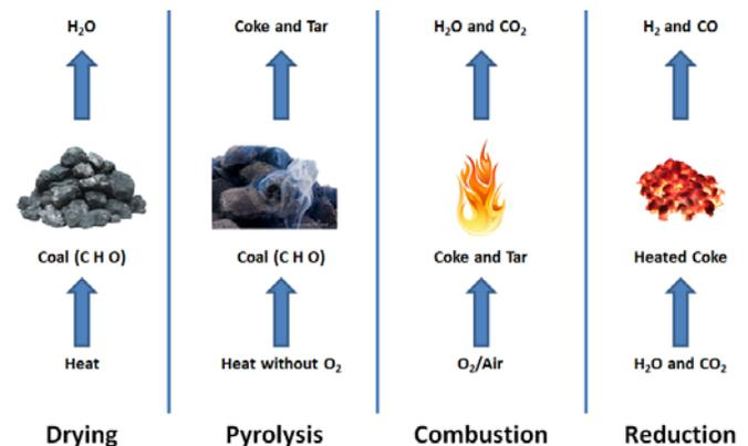
Fig. 1 Gasification Processes
