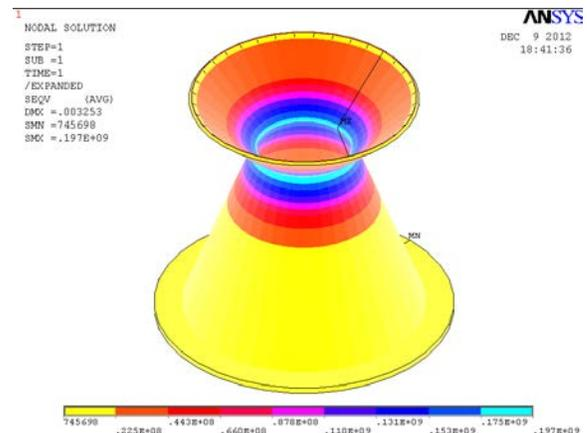
Fig. 9 Von Mises' Stress Distribution in Complete Hearth
