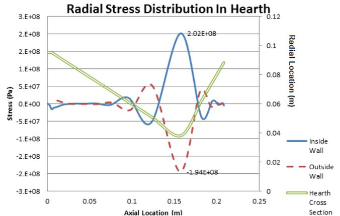
Fig. 12 Radial Stress Distribution in Hearth
