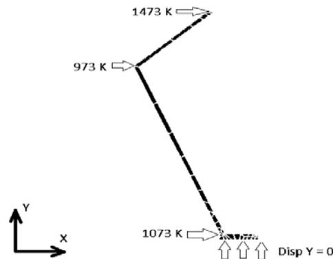
Fig. 5 Meshed Area with Temperature and Boundary Condition
