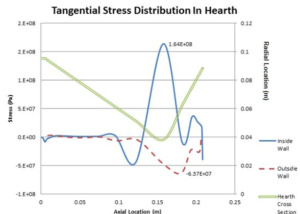
Fig. 14 Tangential Stress Distribution from FEA
