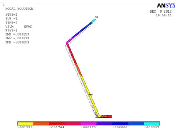
Fig. 7 Displacement vector sum with original geometry
