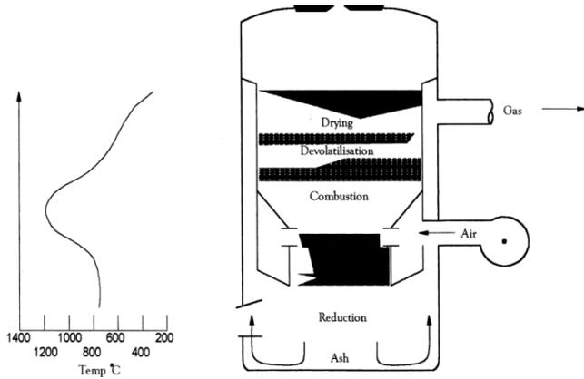
Fig. 3 Temperature Profile of Downdraft Gasifier [8]
