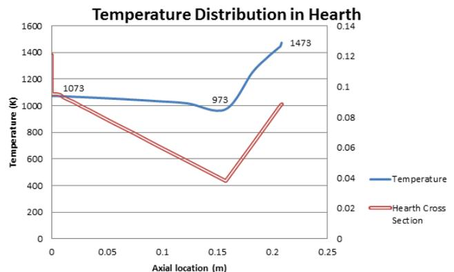
Fig. 10 Temperature distribution in Hearth
