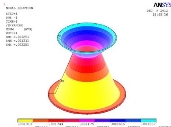
Fig. 8 Displacement vector sum of complete hearth
