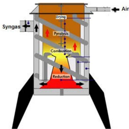
Fig. 2 Downdraft Gasifier
