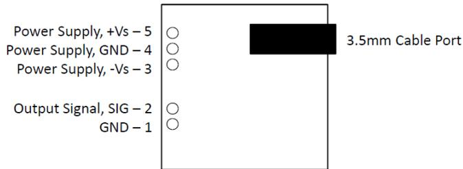
Fig. 3 Pin mapping of muscle sensor.
