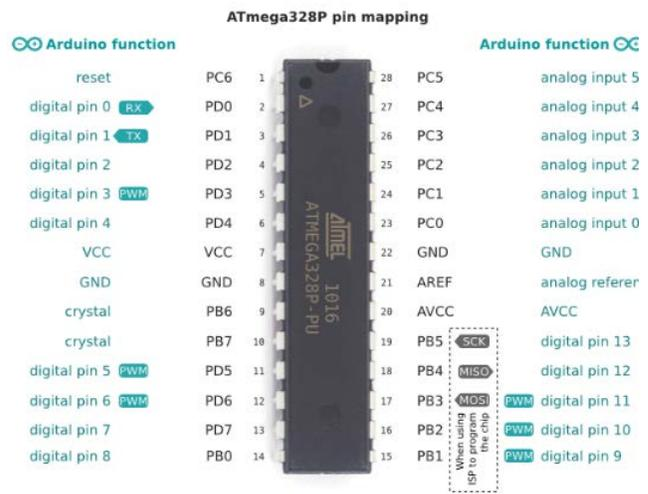
Fig. 4 Arduino Atmega328P pin mapping
