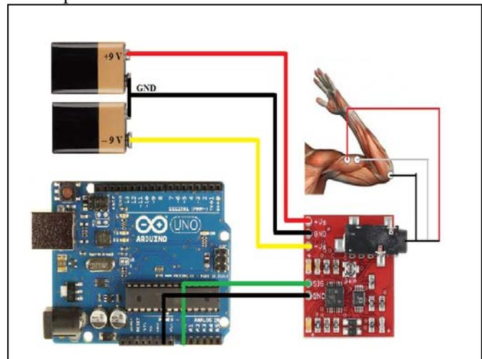
Fig. 5 Circuit diagram of retrieving EMG signal
