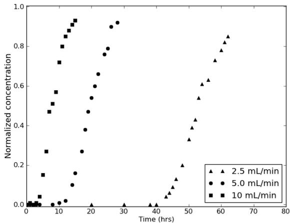
Fig. 2 Effect of flowrate on breakthrough curve for the adsorption of RR2 dye from aqueous solution onto ZPC-10
