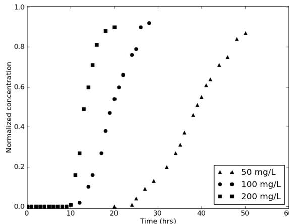
Fig. 3 Effect of initial concentration on breakthrough curve for the adsorption of RR2 dye from aqueous solution onto ZPC-10
