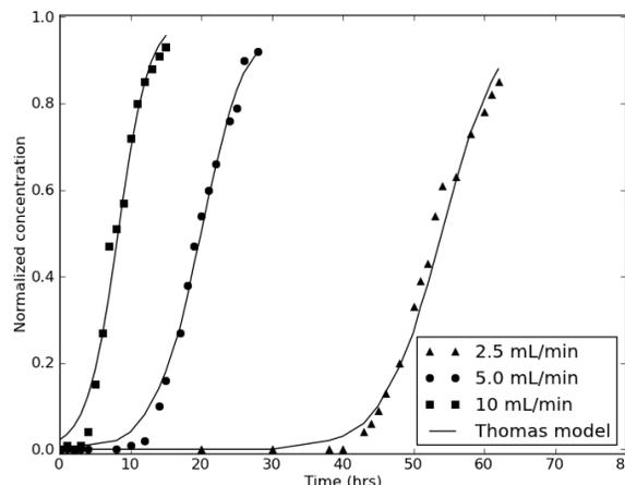
Fig. 6 Comparison of experimental and theoretical breakthrough curve derived Thomas model for the effect of flowrate
