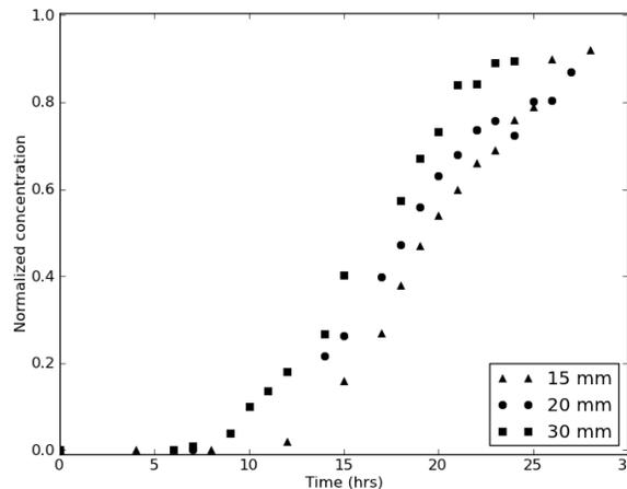
Fig. 4 Effect of column diameter on breakthrough curve for the adsorption of RR2 dye from aqueous solution onto ZPC-10
