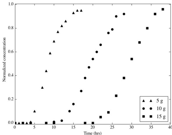
Fig. 1 Effect of bed loading on breakthrough curve for the adsorption of RR2 dye from aqueous solution onto ZPC-10
