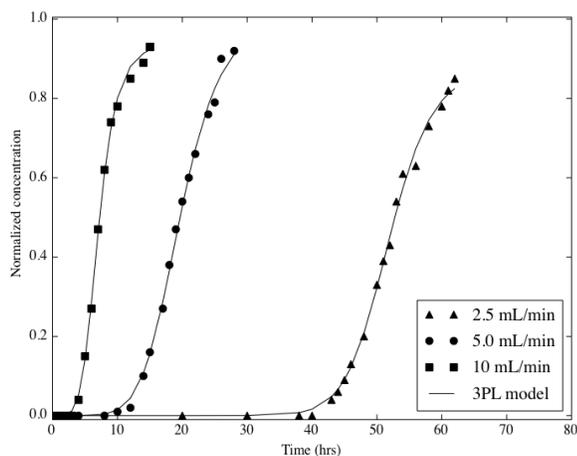
Fig. 5 Comparison of experimental and theoretical breakthrough curve derived logistic parameter model for the effect of flowrate
