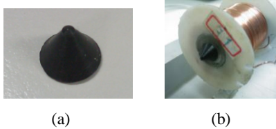
Fig. 16 The prototype of the actuator: (a) The elastomeric cone, (b) The solenoid with the elastomeric cone.
