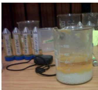
Fig. 1 Formation of various layers during solvent extraction
