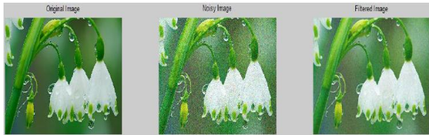
Fig. 5_9 Comparing between median filter, average filter with noise ratio (0.1) on the type of noise 'Gaussian' flower2.jpg . Image with ratio of noise (0.1) 'Gaussian' a) Image filtered by median (3x3) filter. b) Image filtered by average filter.
