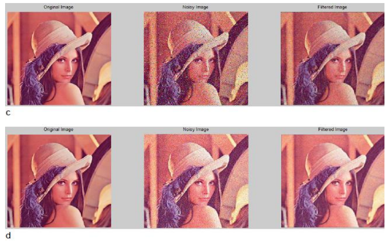
Fig.3_12 Comparing between (salt & pepper and Gaussian) noise lenna.jpg a) Median filter with salt & pepper noise. b) Median filter with Gaussian noise. c) Average filter with salt & pepper noise. d) Average filter with Gaussian noise
