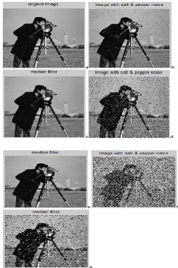
Fig.5.1 Comparing between the ratio of noise 'salt & pepper' with median (3x3) filter cameraman. If a) Original image. b) Image with noise (0.01). And c) Image after median filter. d) Image with noise (0.1). And e) Image after median filter. f) Image with noise (0.5). And g) Image after median filter
