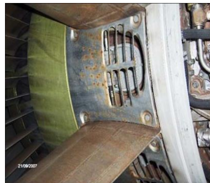
Fig. 7 Pitting corrosion on the engine
