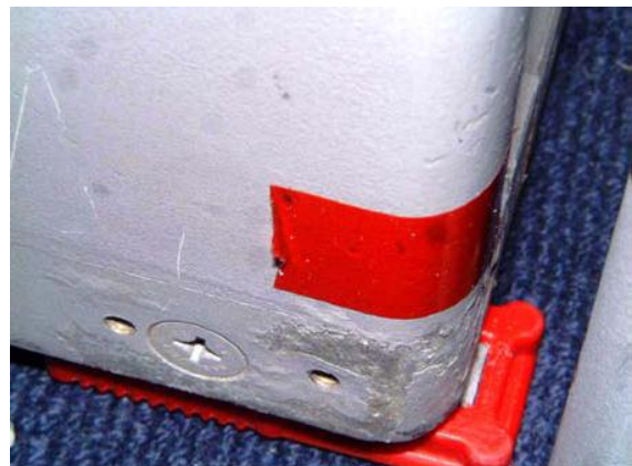
Fig. 8 Exfoliating corrosion at the base of a cabin attendant seat
