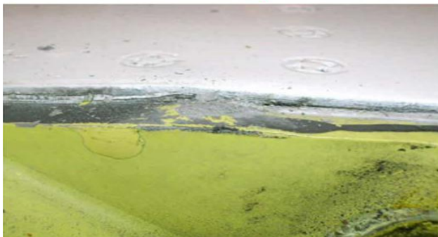
Fig. 4 Exfoliating corrosion on the fuselage
