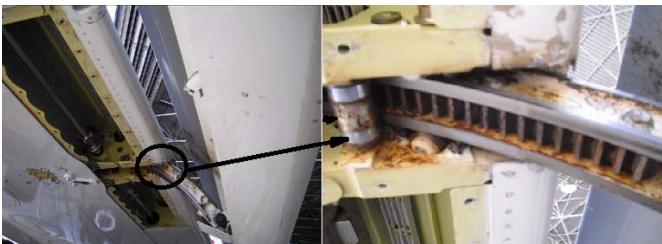
Fig. 5 Atmospheric corrosion on lower wing
