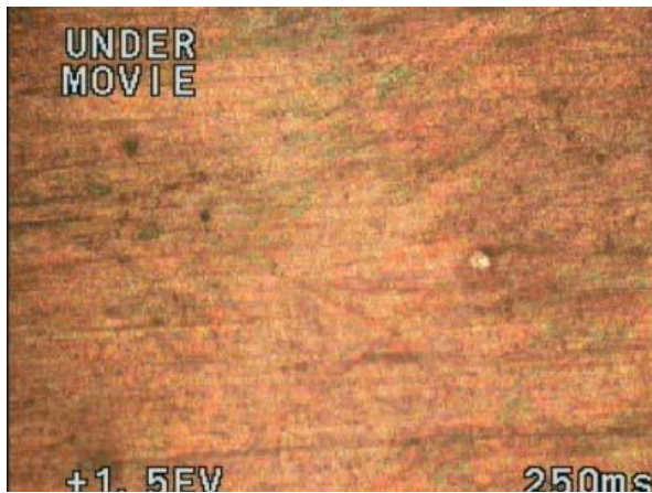
Fig. 13 Aluminium surface after 60 days immersion in sea water.
