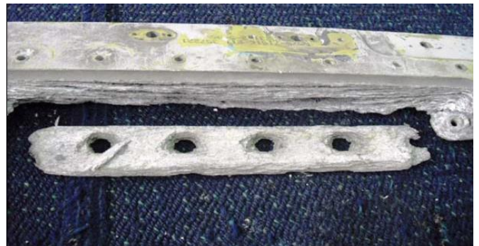
Fig. 2 Badly affected wing flap which resulted in the replacement of the part.
