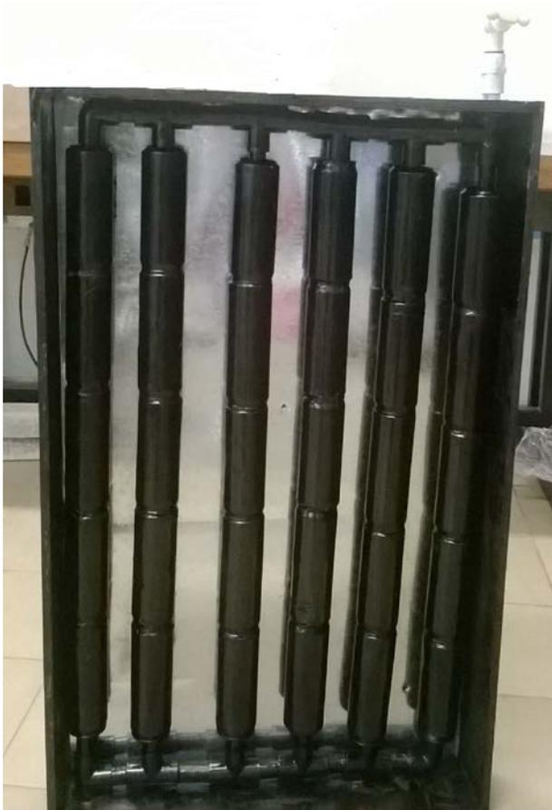
Fig. 7 Working model of SWH system made up of cold drink cans
