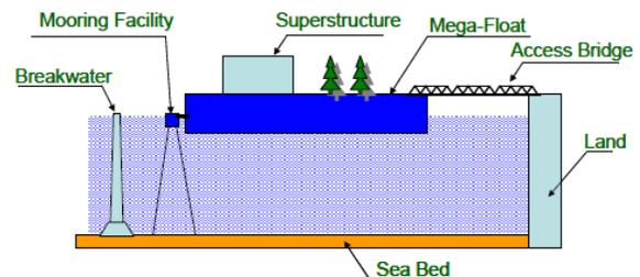
Fig.1 The components of a mega float system which is a large pontoon system Source: (Watanabe, E., etal: 2004)
