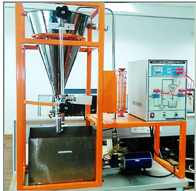
Fig.1 Experimental Setup of Conical Tank Level Process
