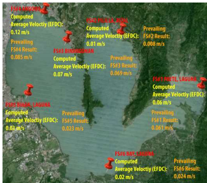
Figure 6 EFDC Velocity Results vs Prevailing Field Survey Result
