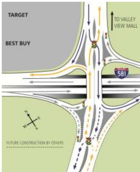
Fig. 1: Valley View Diverging Diamond Interchange Concept, State of Virginia, United States.
