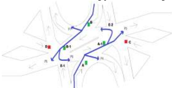
Fig. 7: Blue lines shows the path, green box indicates that traffic signal is open and red box indicates that traffic signal is close.
