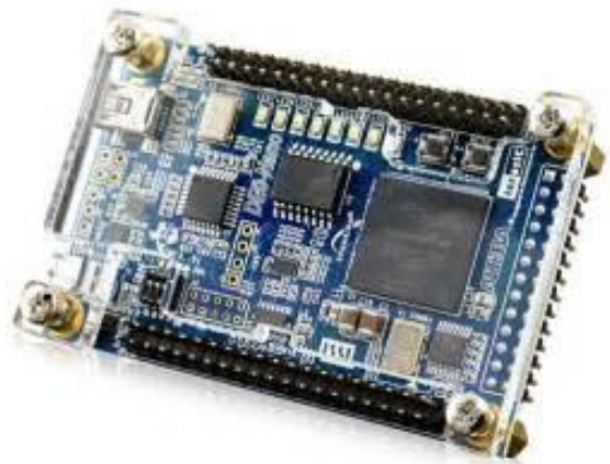
Fig. 2 DE0-nano used for hardware system design
