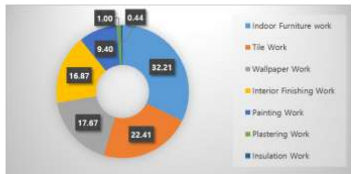
Fig. 2. Status of finish work defect
