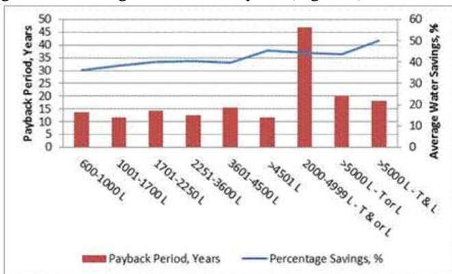
Fig. 1: Payback periods (Years) for different rainwater tank sizes to the households and the corresponding percentage of water saved
