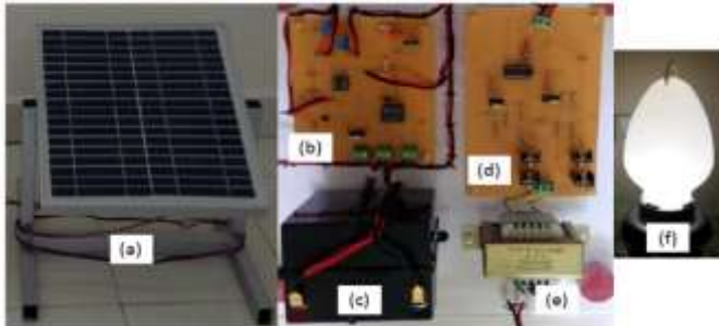
Fig 4: (a) Solar Panel (b) solar charger circuit (c) Battery (d) Push pull inverter (e) Centre tap transformer (f) AC load (3W LED lamp)
