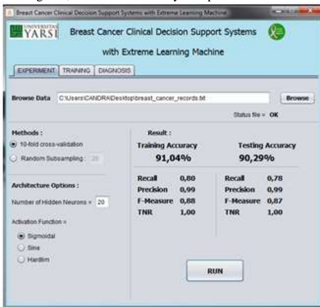
Fig. 1: Experiment subsystems in Breast Cancer Clinical Decision Support Systems. Given patient records, using 10-fold cross validation, 20 hidden neuron, and sigmoid activation function, the systems achieve 90.29% testing accuracy.
