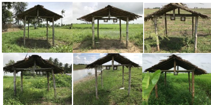
Fig. 2. Installation of Dry Gauze in the Sample House at Difference Distance
