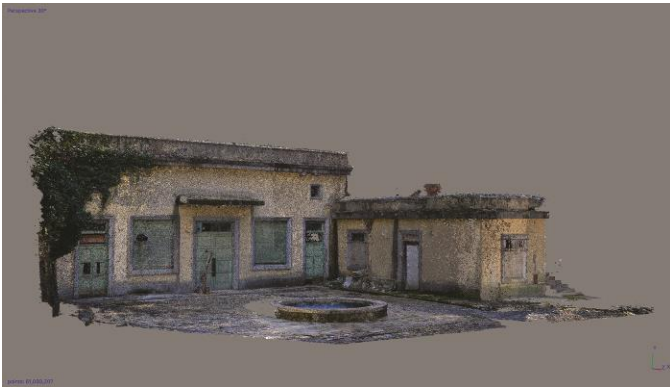
Fig. 5: Digital survey for the creation of the model. Frontal point cloud of the projecting body.
