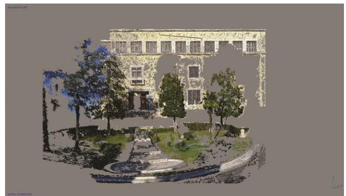
Fig. 1: Digital survey aimed at creating the model. Cloud of the points of the structure and the square in front.
