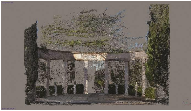
Fig. 3: Digital survey to create the model. Cloud of the points of the structure and of the vegetation system.
