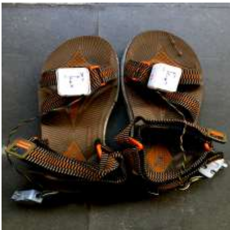
Fig. 2. Shoes with tri-axial accelerometers, 8 membrane switches, X-bee modules located inside the sole
