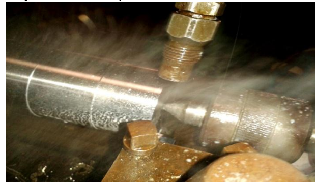
Fig.1. Minimum Quantity Lubrication(MQL)
