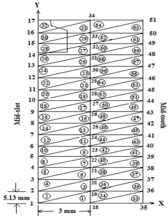
Fig.1. Slice of armature iron and winding bounded by planes at mid-slot, mid-tooth divided into triangular-shaped finite elements.
