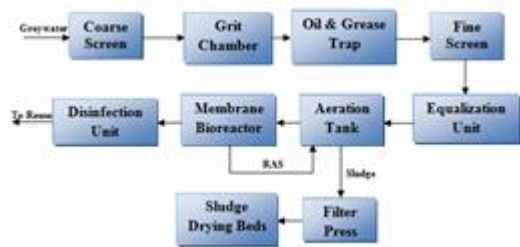
Fig. 3. Schematic Flow Diagram Of Membrane Bioreactor-Based Greywater Treatment Unit.
