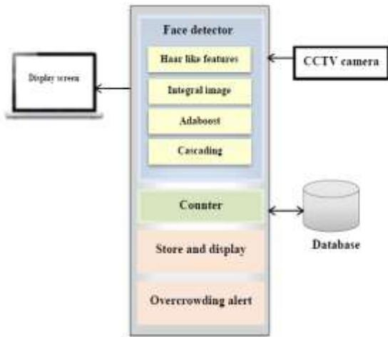
Fig. 1. System architecture and the main system components.
