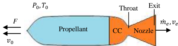
Fig.3. Thrust generation principle of a rocket
