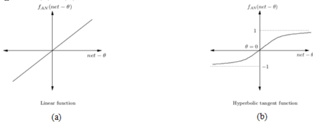
Fig. 2. Activation Functions: (a) Linear function; (b) Hyperbolic tangent function.
