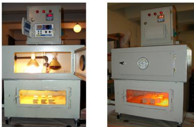
Fig. 2. UV factor and infra red factor of the Preservative's Performance Test Device (S.O.Hattap)
