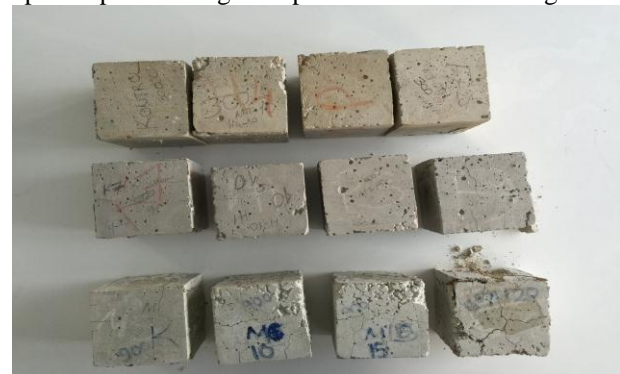
Fig. 3. Concrete samples exposed to high temperature
