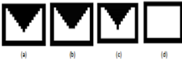
Fig. 5: Convex hull detection of concave image (98x99) . (a) input image, (b) result of the execution rule 5, (c) result of the execution rule 8, (d) result using a best packet of CA with 8 iterations and 5.4966 sec
