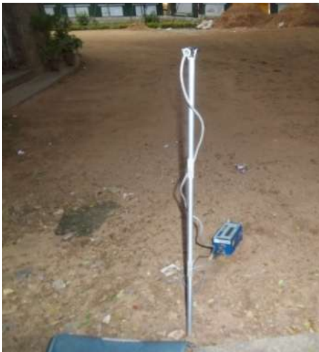
Fig. 4 Ground Vibrations Monitoring near the Structures
