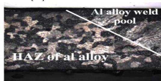
Fig. 12 Grain at Heat affected zone of aluminum alloy [13]
