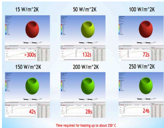
Fig.3 Control simulation results using different film coefficient
